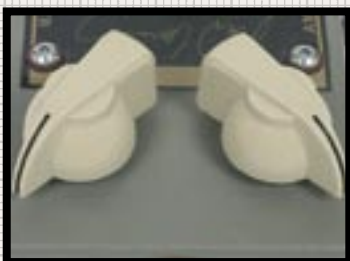
■ The Fat TB's controls offer continuous travel, while the V2's is stepped
